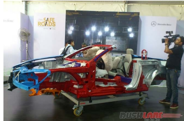
Picture 4. Body-in-white model, incl. airbags and sensors
