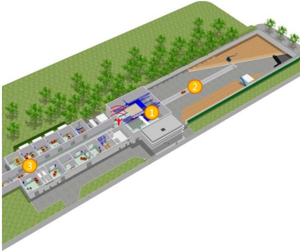
Figure 3. Laboratory Setup: 1- Impact area; 2- outside area; 3- acceleration tunnel
