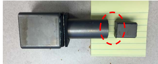
Figure 18 Failure of THOR-50M femur plunger shaft The knee design is the same as THOR-50M.
