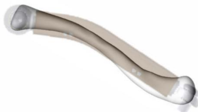
Figure 6. Overlay of THOR-05F clavicle and statistical shape model defined in Lu et al 2013.
