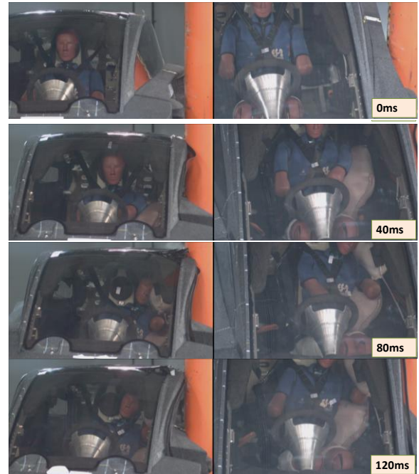
Figure C-2. Dummy kinematics in Pole crash test.
