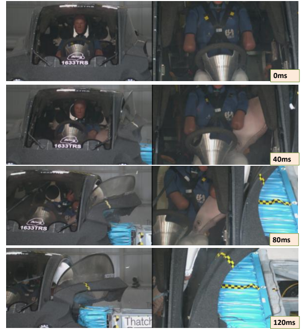
Figure C-1. Dummy kinematics in MDB crash test.
