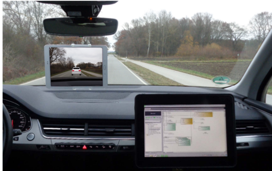
Figure 2. Integration of the ViL test system into a real test vehicle
