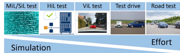
Figure 7. The ViL test method closes the gap between simulated and real-world tests
