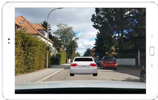
Figure 4. Within the AR display crash opponents are placed into the real test environment
