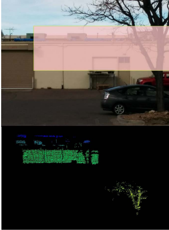
Figure 10. TOP) Target scene with a large wall 180 ft away. Far back wall is 285ft away. BOTTOM) LiDAR image of the same scene. Dark blue is the far wall and the light blue are the AC units mounted on the roof approximately 225ft away.
