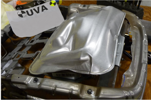
Figure 2. Metal pelvis restraint cushion (PRC) in the front seat (post test).
