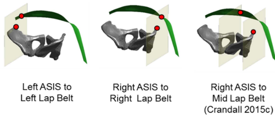
Figure 9. Definitions of measurement points for calculating the submarining distance.
