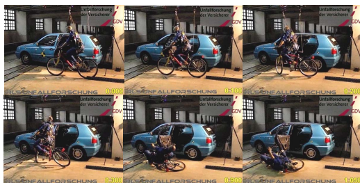
Figure 10: Collision with a driver's door open at an angle of 90 degrees and with an overlap half the length of the handlebar
