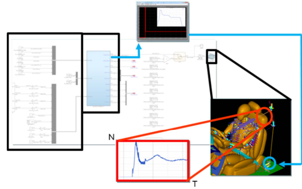
Figure 9. Co-Simulation of ASB (Active Seat Belt) logic and occupant simulation
