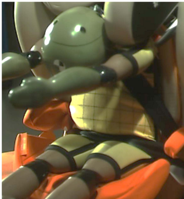
Figure 13. Dummy and diagonal belt interaction
