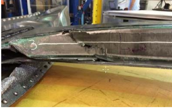
Figure 14. Crushing of Hat Section.
