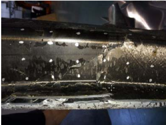
Figure 15. Debonding of Hat and Spine.
