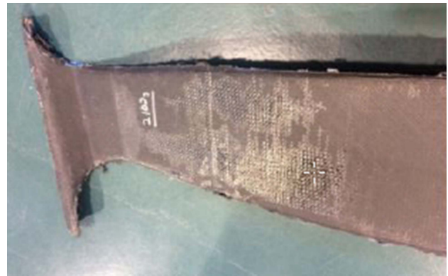
Figure 7. Dry-Spots after Infusion.
