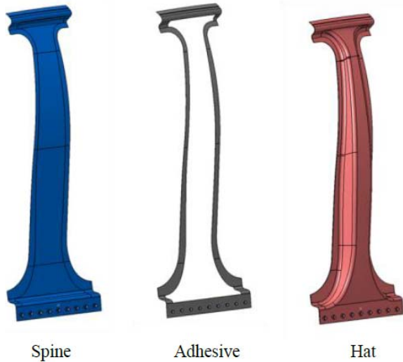
Figure 2. Spine-Hat Adhesively Bonded Composite B-pillar.
