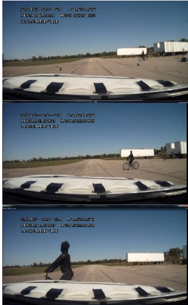
Figure 10. Surrogate bicyclist crash test when crossing road
