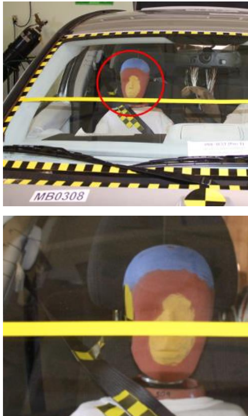
Figure 1. Shoulder belt routing of small female right front passenger dummy in official NCAP test of Dodge Caliber
