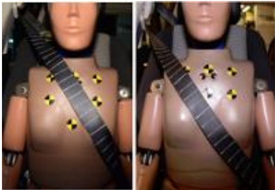
Figure 3. Sled tests of small female dummy, forwardmost seat position: D-ring full-up (left), full-down (right)
