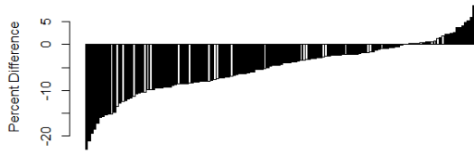
Figure 11. Maximum delta-v percent differences (EDR with respect to instrumentation) for the 140 cases. The black bars show the cases with complete pulses recorded by the EDRs.
