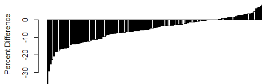
Figure 13. ASI percent differences (EDR with respect to instrumentation) for the 140 cases. The black bars show the cases with complete pulses recorded by the EDRs.
