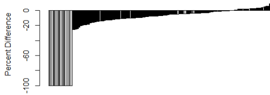
Figure 12. OLC percent differences (EDR with respect to instrumentation) for the 140 cases. The black bars show the cases with complete pulses recorded by the EDRs.
