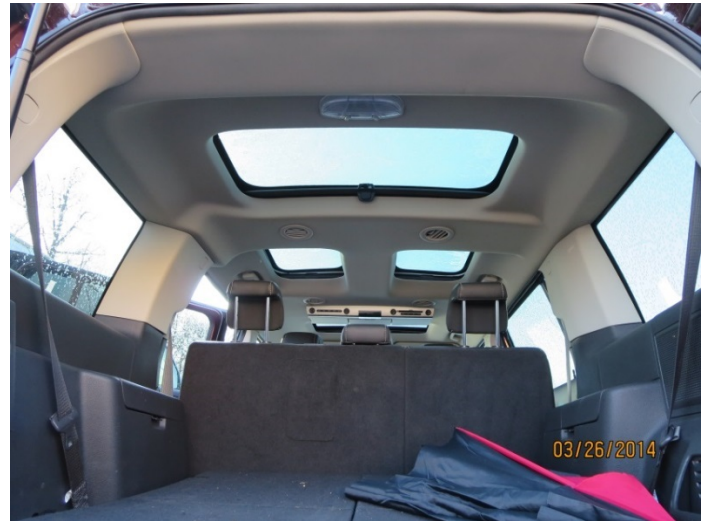
Figure 2 - Ford Flex Interior Showing Three Distinct Daylight Openings
