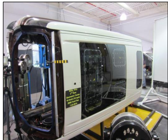
Figure 6 - Vehicle Prepared to Accommodate the Ejection Impactor
