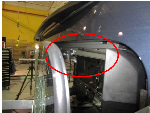
Figure 14 - Typical Failure Mode at the Rail for the Movable Glass Panel
