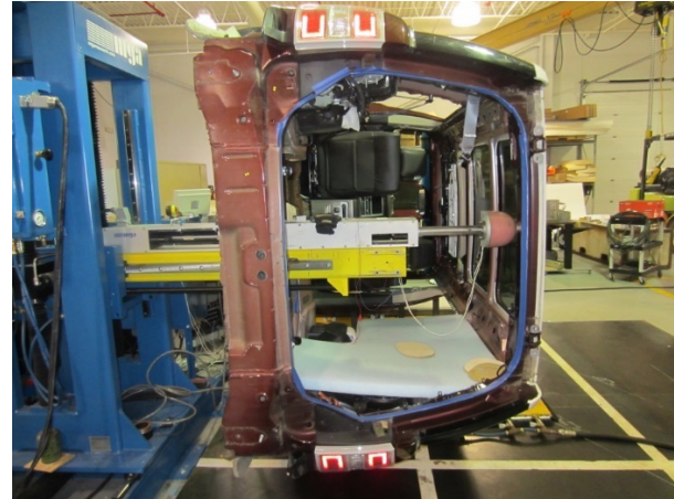
Figure 11 - Typical Setup for Ejection Impacts
