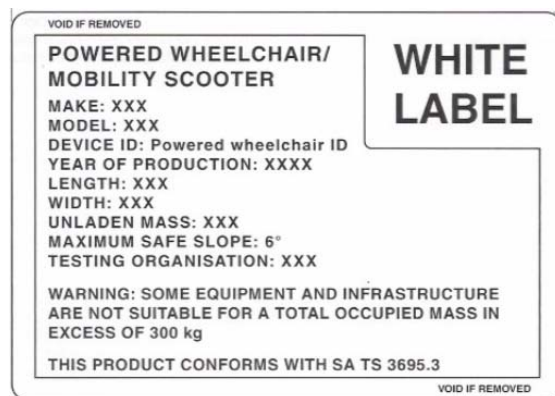
Figure 4. White Label for footpath use (© Standards Australia)
