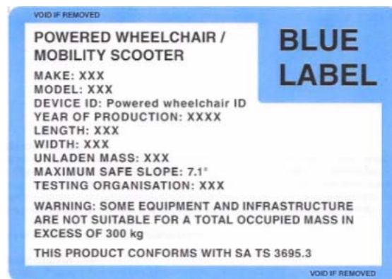
Figure 5. Blue Label for compatibility with suitable public passenger vehicles (© Standards Australia)
