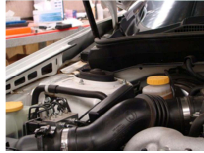
Recent: Firewall and sides of engine bay lowered with bonnet supported by collapsible elements. Suitable clearance is provided between suspension tower/other under bonnet structures and bonnet.
