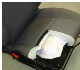
Figure 7: Pelvis restraint cushion in a front seat.
