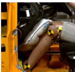
Figure 6: Inflated knee airbag in a frontal sled test.
