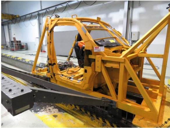
Figure 2: Body in White used for occupant sled tests with the THOR dummy
