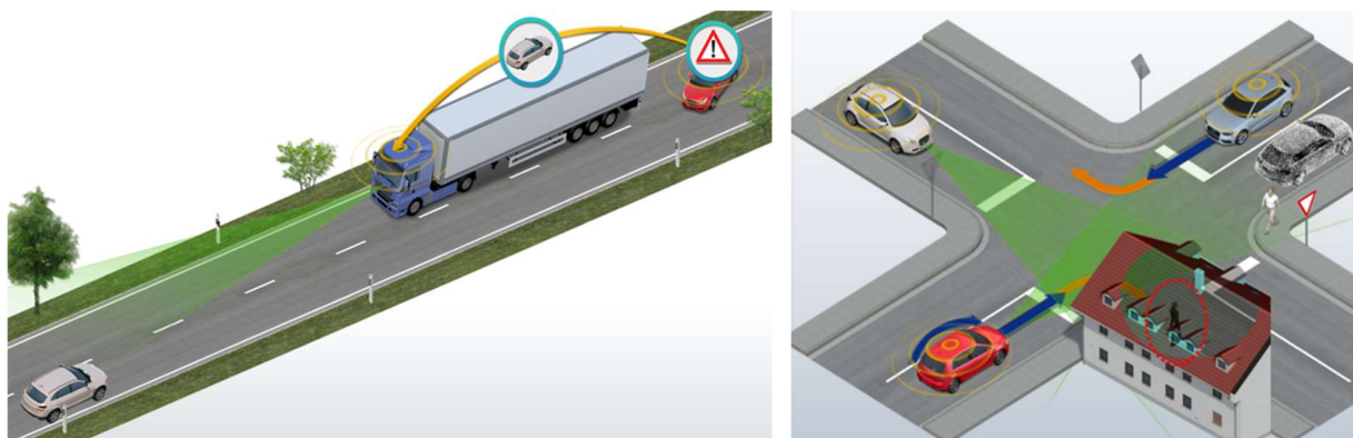
Figure 2: Left: Truck sends information to red vehicle regarding non-V2X-equipped white vehicle. Right: White vehicle sends information to red vehicle regarding NLOS VRU [6].
