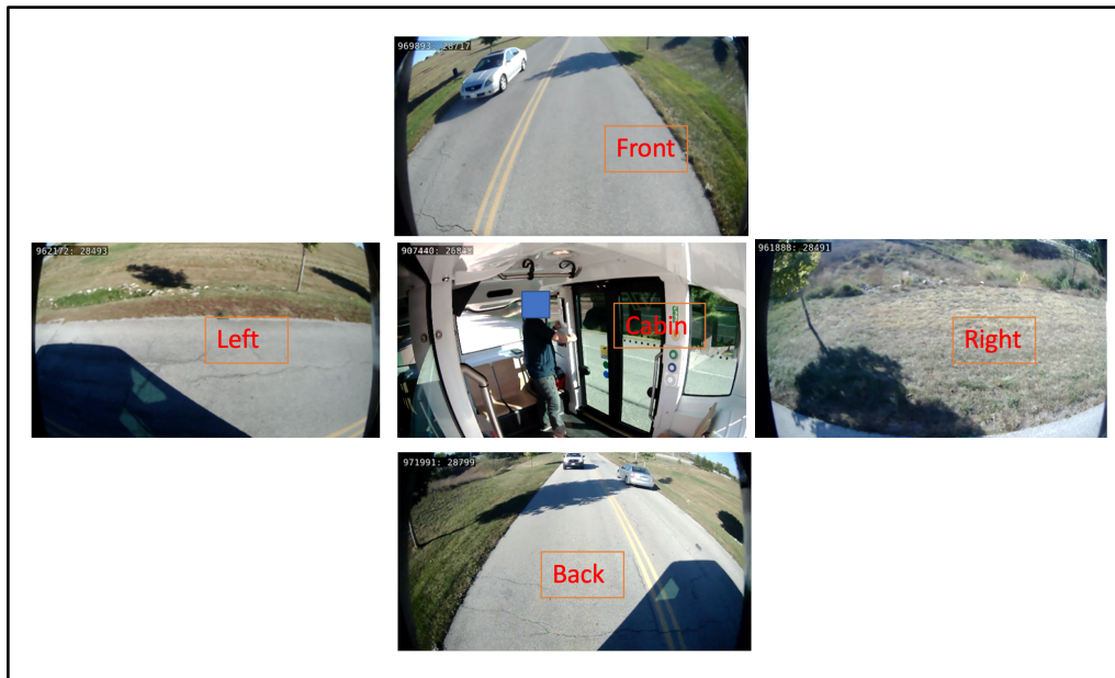
Figure 2. Video images. Example of scene cameras capturing 360-degree information around the LSAV.
