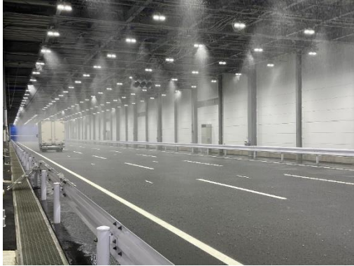
Fig.10 Rainfall in specific environment test facility
