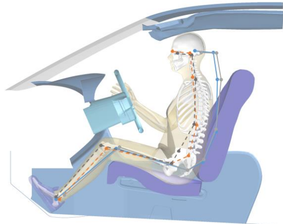
Figure A2. Comparison of model postures based on the regression model by Park et al. (2016) with the 50F model. The orange dashed lines illustrate the posture achieved for the 50F model. As a reference, the posture prediction for the 50F occupant is shown in dashed grey lines. The torso of the 50F model was repositioned slightly from the initial posture in order to better match the predicted head position. Note that the regression model predicts a knee position which is not achievable with the femur length in the present model.
