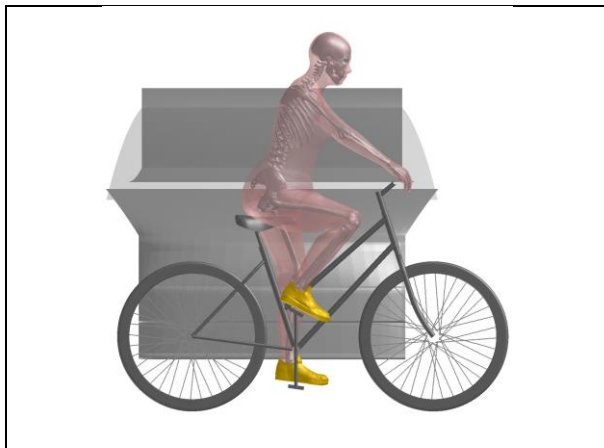
Figure A9. Positioned 50F cyclist model in front of GV sedan model
