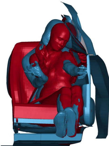
Figure B6. Overlay of 50F (red) and 50M (blue) VIVA+ model response for near-side impact (ID 5) 70 ms into the simulation.
