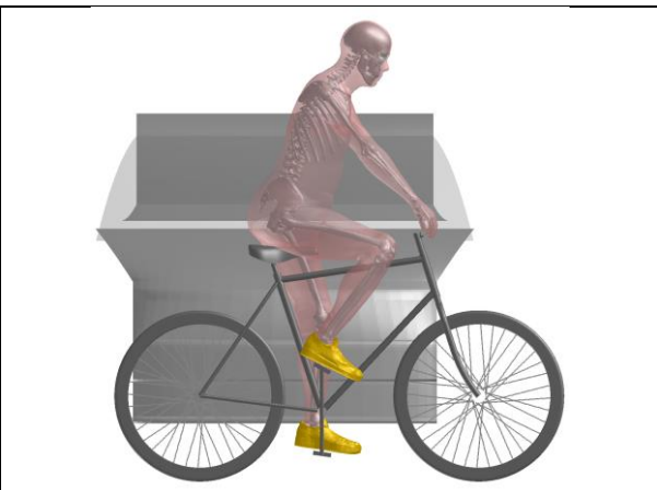
Figure A10. Positioned 50M cyclist model in front of GV sedan model
