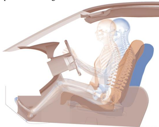
Figure 1. Comparison of the final postures of the 50F (orange) and the 50M (blue). Note that the same eye level was achieved and both occupants can reach the pedals as well as the steering wheel.
