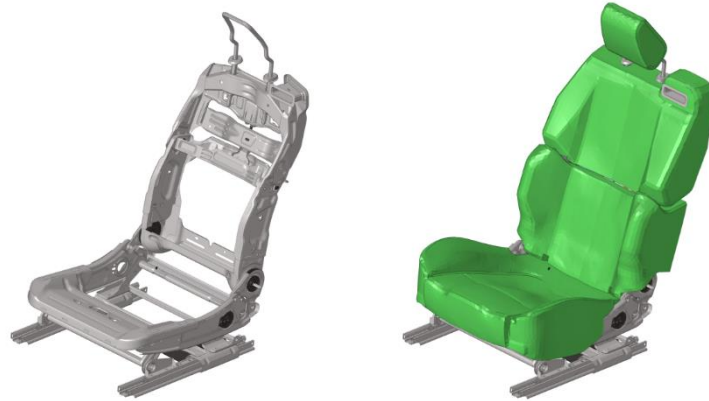
Figure 2. Conceptual orvia innovation seat used for rear impact simulations
