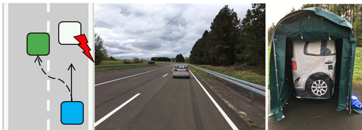
Figure 2. Left: Schematic overview of the cut-out maneuver performed by the lead vehicle (green) in front of the stationary crash target (white). Center, Right: The target is hidden in a tent and not visible for participants prior to the test scenario, where it is placed in the center of the driving lane by a third experimenter.
