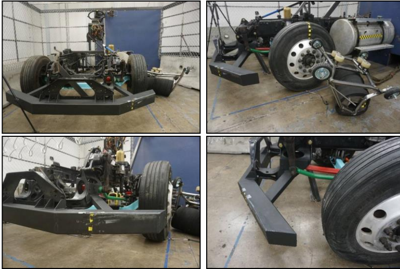
Figure 14. FUPS Sled Post-Test Photographs
