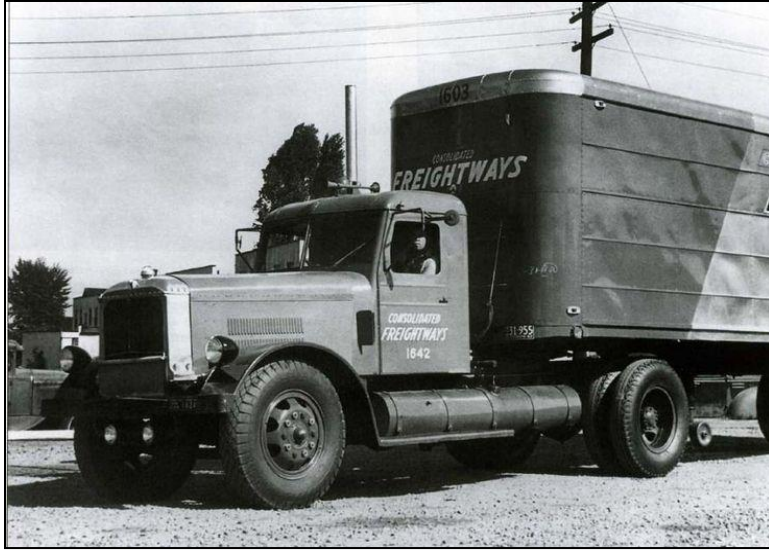
Figure 1. Consolidated Freightways Truck (Precursor to Freightliner) Fuel Tank Placement
