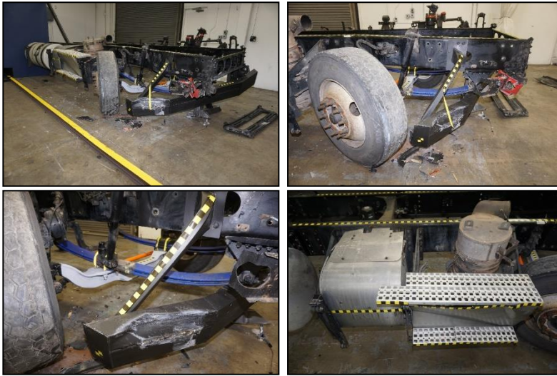
Figure 7. FUPS Sled Post-Test Photographs
