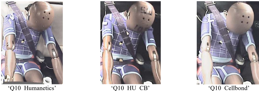
Figure 10. The shoulder-belt to shoulder interaction of the three different versions of Q10 at the time of max forward excursion in a frontal impact.
