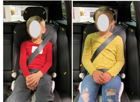
Figure 4b. Two children trying out the booster prototype in Jakobsson et al. (2020). The shoulder-belt is routed under the belt guide for the 6-year-old (left), while over the belt guide for the 11-year-old (right).
