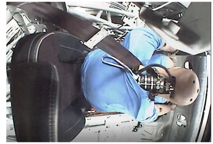
Figure 8c. Top view of shoulder-belt interaction with Humanetics updated THOR-50M shoulder pad, during frontal impact.
