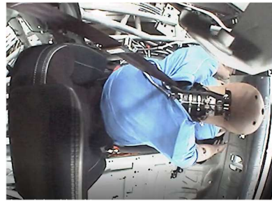
Figure 8b. Top view of shoulder-belt interaction with the original THOR-50M shoulder pad, during frontal impact.
