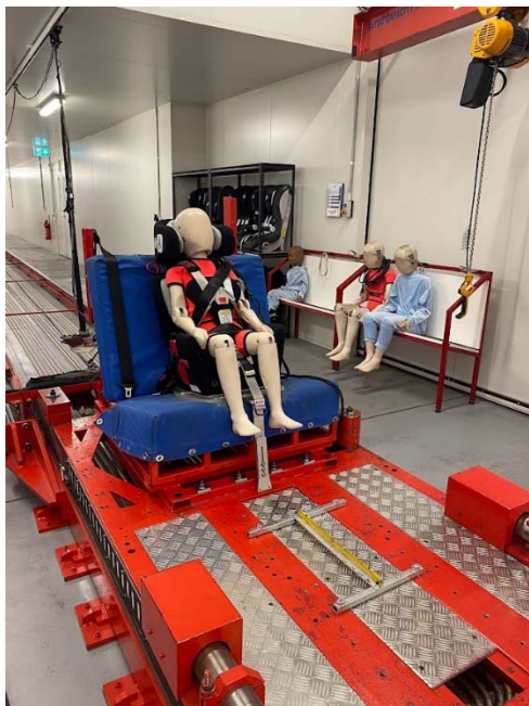
Image 1. Carrot 3000 set-up for testing at Britax Childcare Pty Ltd, Australia.
