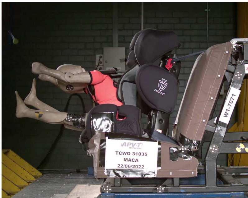
Image 5. Frontal test resulting in splitter plate breakage.
