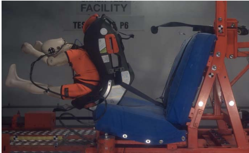
Image 4. LATCH and top tether failure.
