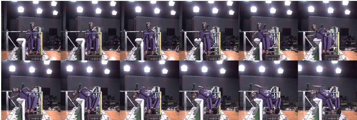
Figure 5. The image sequence shows a full dummy sled test.
