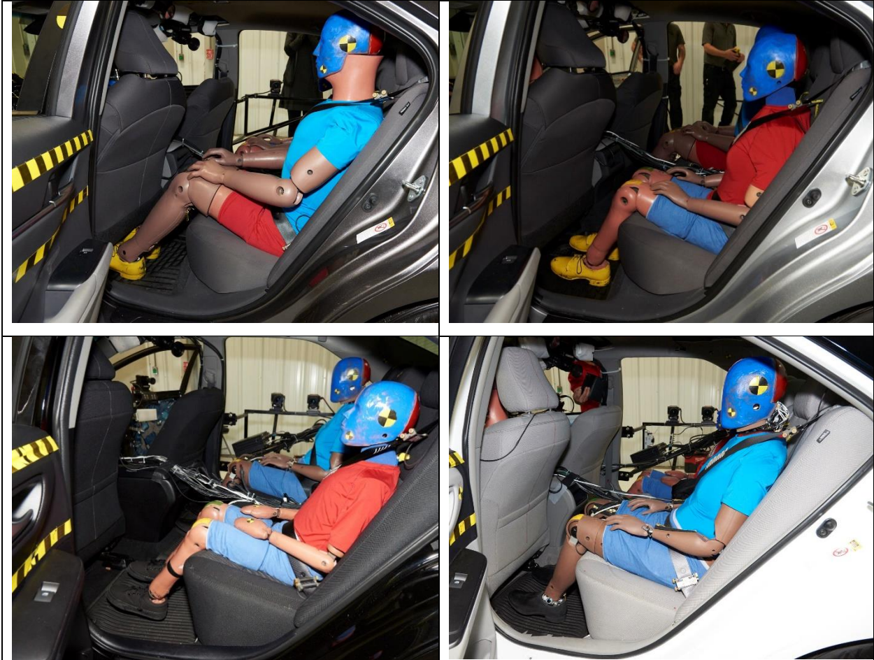
Figure 2. ATDs seated in left rear seating position, H3-50M (top left), H3-5F (top right), H3-10YO (bottom left), THOR-5F (bottom right).
