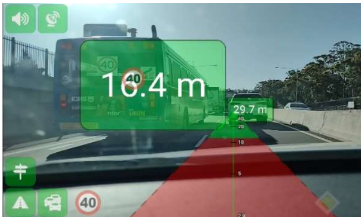
Figure 6. Screenshot from screen capture of UGV Driver Assistant (Android) detection of 40km/h sign on rear of bus (40km/h zone not active).
