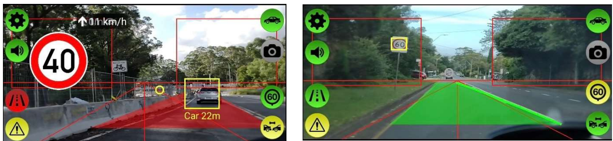
a b Figure 1 a & b. Screenshot from screen capture of aCoDriver App (Android). a) Speed zone reminder (40), LDW, FDW. b) Speed zone detection (60), Lane path OK, centerline detection.
