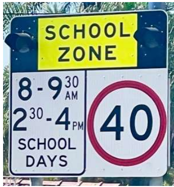
Figure 3. Australian time dependent School Zone sign. 40km/h limit applies during listed times.
