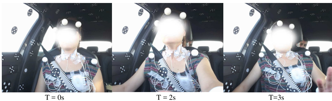
Figure 18: Video sequence analysis of volunteer n.3: left = relaxed, middle = neck activation + forward movement, right = trunk activation + rearward movement
