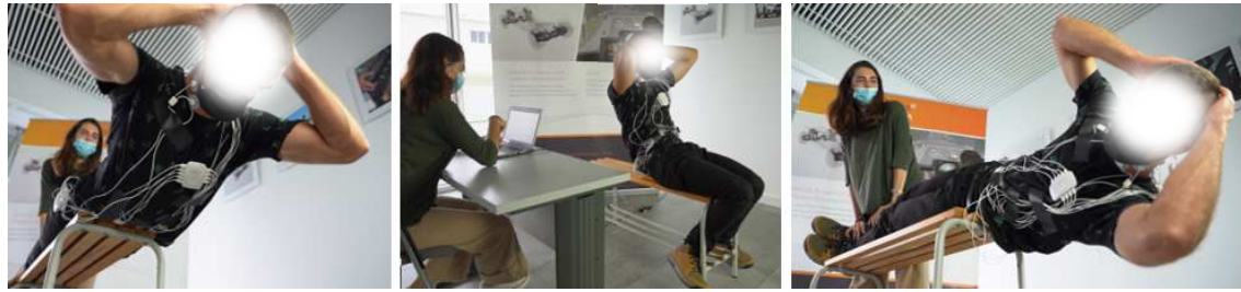
Figure 10: Calibration exercise for MVC of rectus abdominis (a), obliquus externus (b) and erector spinae (c)
