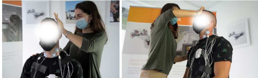
Figure 11: Calibration exercises for MVC of splenius capitis, splenius cervicis, sternocleidomastoid and scalenus
