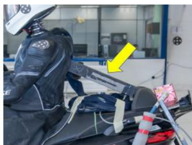
Figure 5. Foam block used to increase stability during the crash
