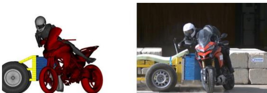
Figure 14. Impact with airbags: front view at 74ms
