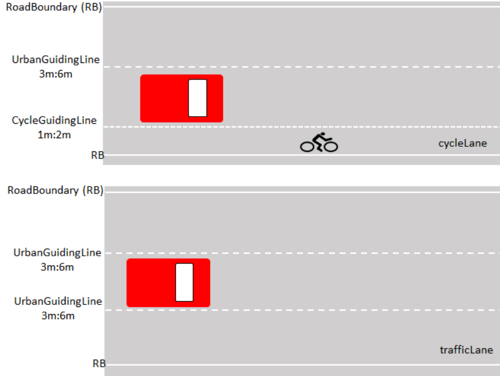
Figure 11. Ego Lanes left connected to the Urban Guiding Lines and right connected to the Cycle Guiding Line (top), and right connected to the Urban Guiding Line (bottom).
