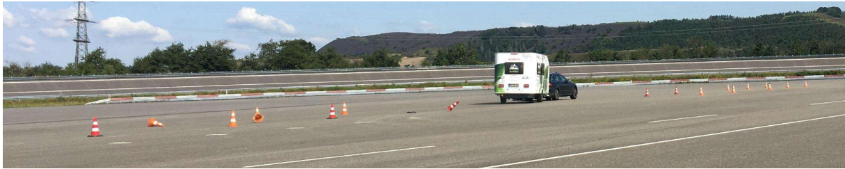
Figure 2: Non-valid test run in double lane change test
