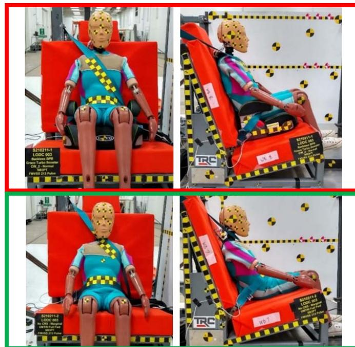
**Figure 1. LODC seated on FMVSS No. 213 bench<sup>1</sup> with BPB (top) and slouch position without BPB (bottom).**
