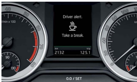
Figure 2 – A typical indirect driver status monitoring output (Škoda)
