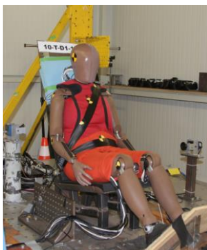
Figure 1. Sled test setup: Rigid seat, 3-point belt system with shoulder belt pretensioner and load limiter
