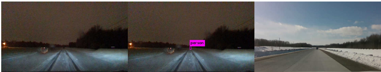
Figure 8. DNN-based object recognition and classification demonstrated irregular performance (left: input image from test conducted at night, middle: relevant objects detected and classified in the left image, right: detection failed even in sunny conditions).
