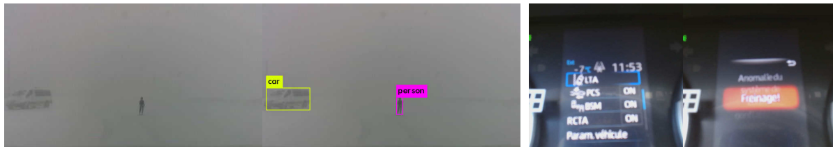
(a) YOLOv3 DNN model detecting and classifying target objects (left:input, right: output), (b) Instrument cluster transitioning from normal state to AEB warning state.
