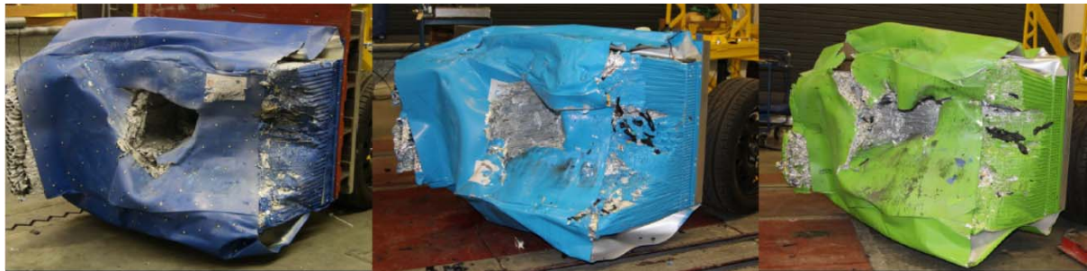
Figure 8: Comparative test MPDB face deformation
