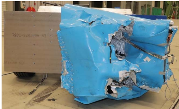
Kerb mass: 2173kg Deformation SD: 172mm Bottoming out: Yes
