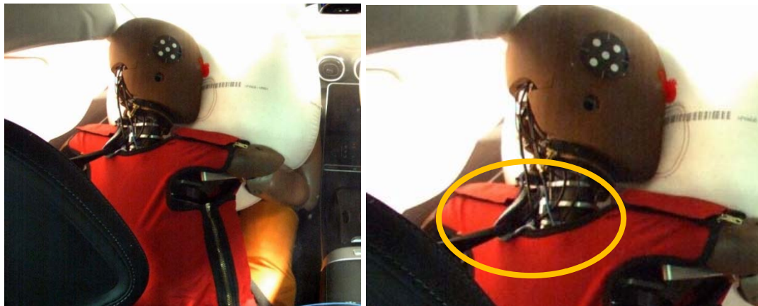
Figure 10: THOR diagonal belt slippage
