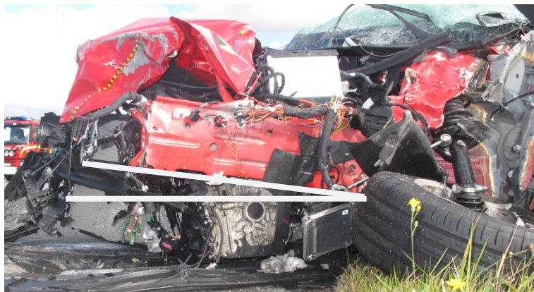
Figure 16: Front Longitudinal Deformation and Apparent Upward Rotation
