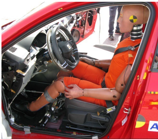
Figure 3. Driver position - note position of right foot.
