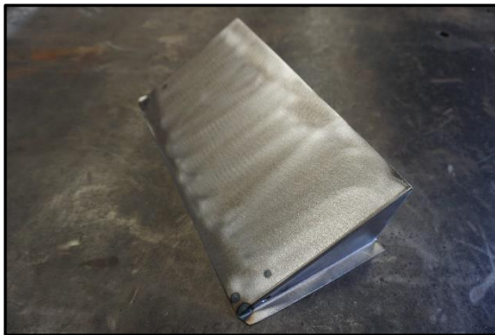
Figure 16: Improved Design – Diverter Shield
