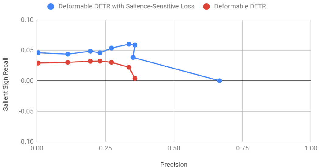
Figure 7. How well does the Saliency-Sensitive Loss bring out performance on salient signs? In this graph, we show the difference in performance between salient sign recall and all sign recall (in other words, how much better is the model at recalling salient signs than the aggregate collection of signs). Deformable DETR does generally perform better on salient signs than all signs together, but with exception as precision increases (in fact, negative at its greatest precision). On the other hand, Deformable DETR with saliency-sensitive focal loss maintains improved performance on salient signs, and at greater margin than the baseline model.
