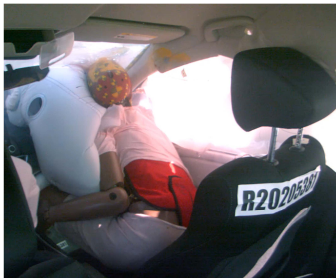
Figure 6. Passenger-side head impact with the windshield in test v11287, right 30° angled (near side), 48 km/hr.
