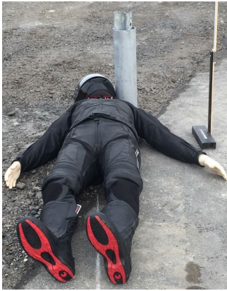
Figure 4: Biofidelic crash test dummy at impact point (sigma post covered with a pipe) (source: BAST)
