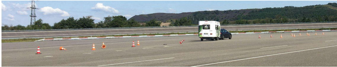
Figure 2: Non-valid test run in double lane change test problems for example is the closed-loop double lane change test.
