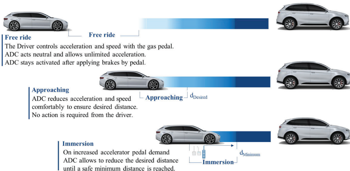
Figure 1: Functional principle of Adaptive Distance Control (ADC)
