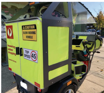
Figure 7. Speed indication sign on a vehicle. Postal service delivery trike (top speed 45km/h).
