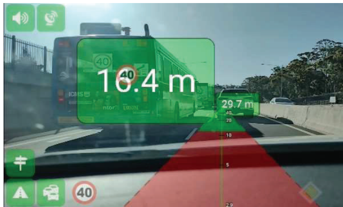
Figure 6. Screenshot from screen capture of UGV Driver Assistant (Android) detection of 40km/h sign on rear of bus (40km/h zone not active).
