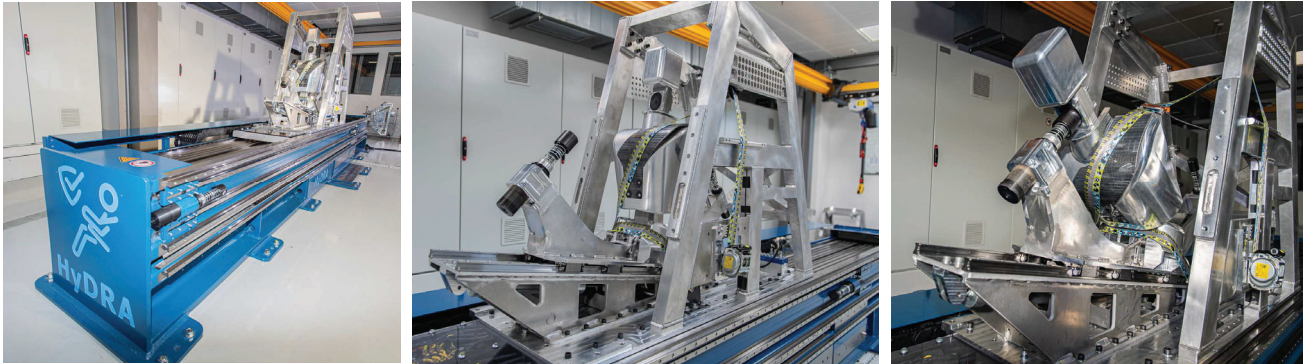
Figure 12 “Rebound Guy Mk I” (RBGI) on HyDRA® (see [10]) test bench (photo left). Close up before the test (photo center) and after the test (photo right). The SBS is fitted on a lightweight aluminum frame structure, designed to represent the PGV vehicle coordinates but it allows also to vary fixation points. Viscous damper with force load cell hidden underneath lower body rail.
