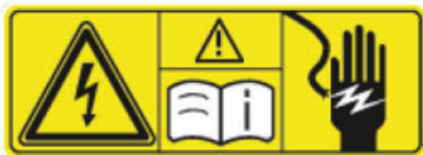
Figure 8: Warning message on HV components
