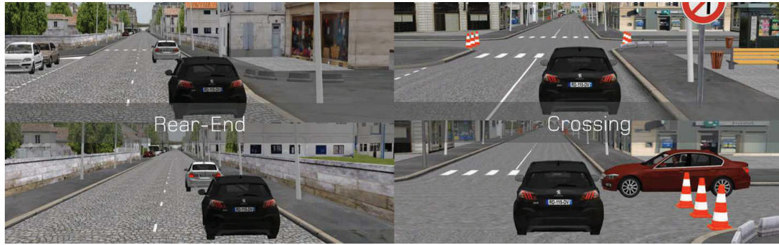
Figure 1: Load cases: rear-end (left; EGO vehicle - black) and crossing (right; EGO vehicle - black)
