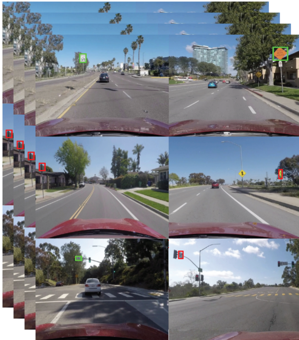
Figure 3. Example Sign Annotations from the LAVA Salient Signs Dataset. A green bounding box indicates a salient sign and a red bounding box indicates a non-salient sign. As shown in the figure, the salient annotations often mean that the sign relates to the current lane or intersection the driver is in and provides meaningful information that affects the driver’s future actions. On the other hand, the non-salient signs are often in a different lane, intersection, or face the wrong way, so these signs don’t offer any important information. A vehicle’s intended maneuver is important in classifying sign salience, so temporal dynamics should be considered when annotating and utilizing salience data, as explained in [2].
