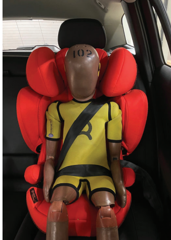
Figure 8b. A booster seat with a 6-year-old-sized ATD in the rear-seat of a modern passenger car.
