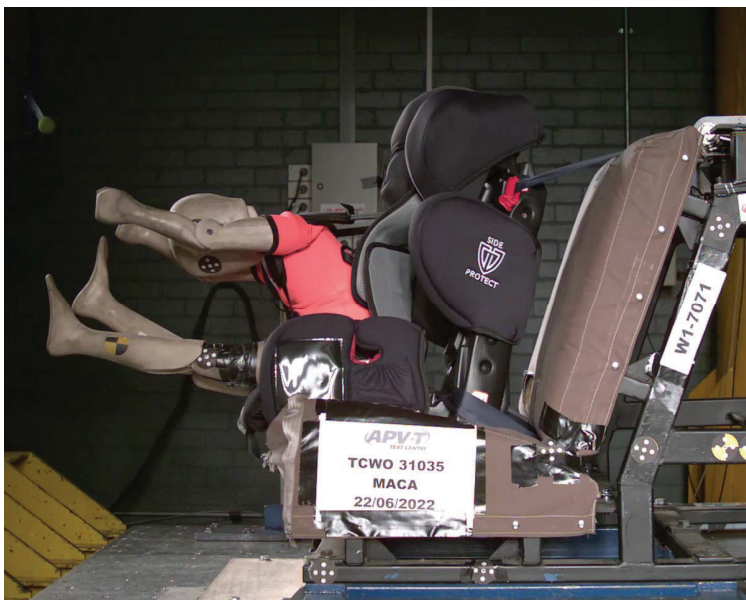
Image 5. Frontal test resulting in splitter plate breakage.
