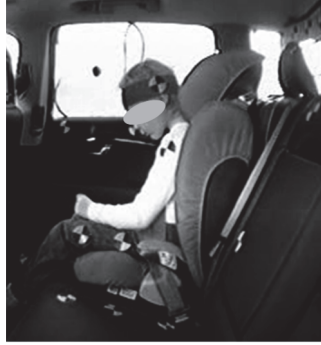
Figure 3a. Maximum forward head position of a child restrained in a booster seat during an emergency braking event (Stockman et al., 2013).
