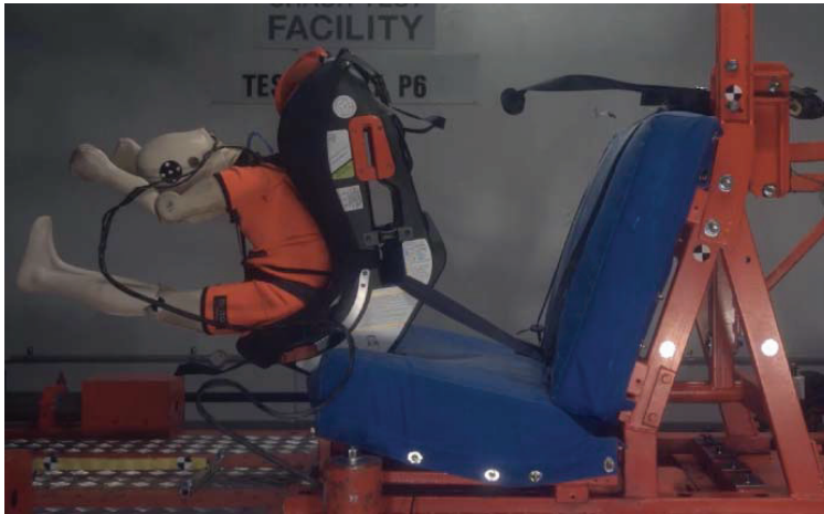
Image 4. LATCH and top tether failure.
