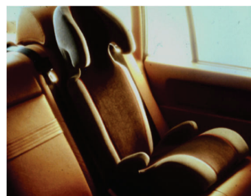
Figure 1c. A booster seat from 1989. As the prior version (Figure 1b), it is a booster seat with removable backrest.
