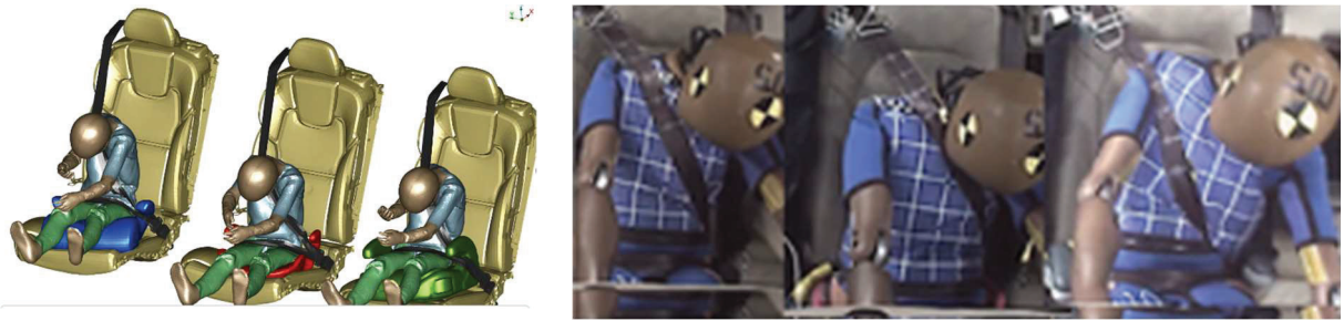
Figure 13. PIPER6y (left) and Q10 (right) at the time of maximum head excursion restrained on three different booster cushions (Bohman et al., 2020b).
