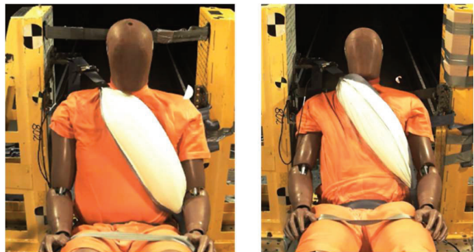
Figure 12b. THOR-50M with a 10 liters air belt, in the sled test setup of upright (left) and reclined (right) seat position.
