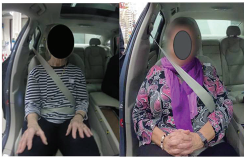
Figure 3a. Examples of passengers with different body constitutions and their beltfit (Osvalder et al., 2019).
