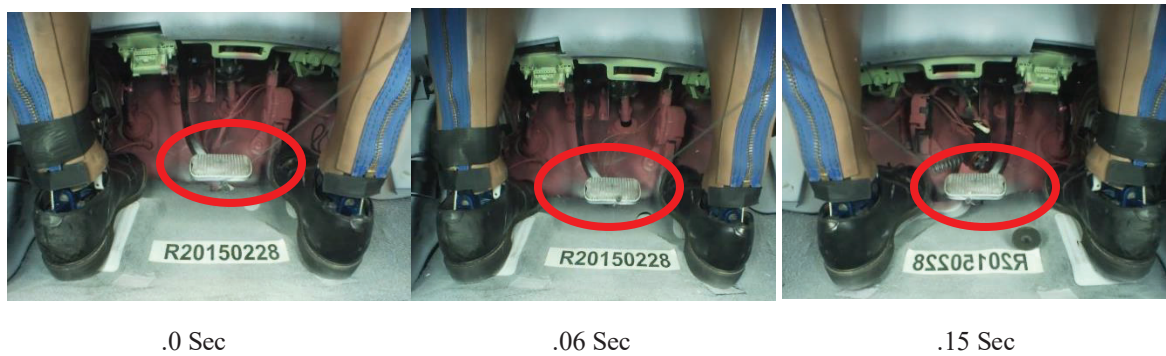
Figure 6a. Brake Pedal Motion in Test 9335; 5 mm Recorded Brake Pedal Intrusion
