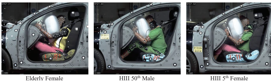
Figure 7. Images of the driver seats taken 80 ms post-impact.
