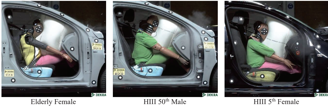
Figure 14. Images of the front passenger seats taken 80 ms post-impact [14].
