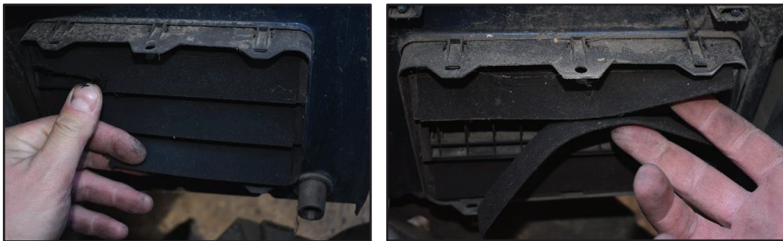
Figure 3: Exhauster vent 4a driver's side (Left) and 4b passenger's side (Right)
