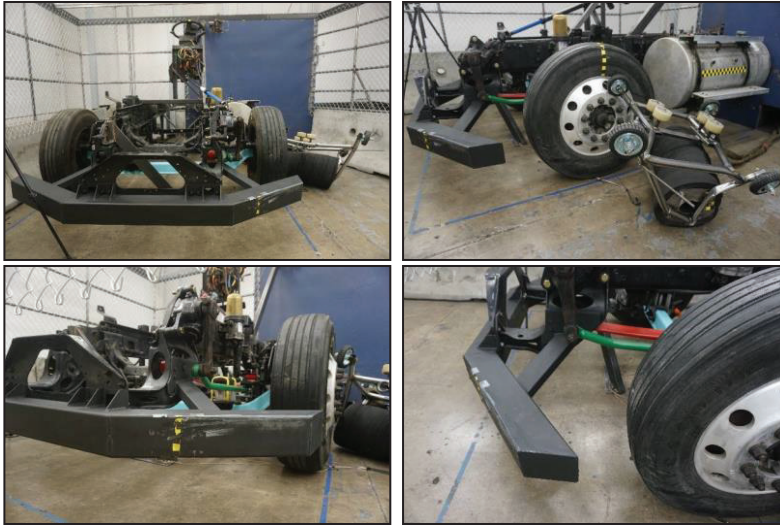
Figure 14. FUPS Sled Post-Test Photographs
