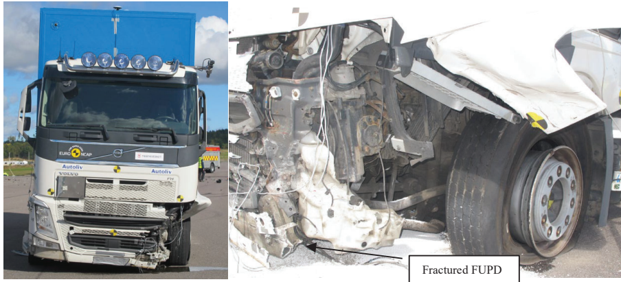
Figure 11. Damage to the HGV.
