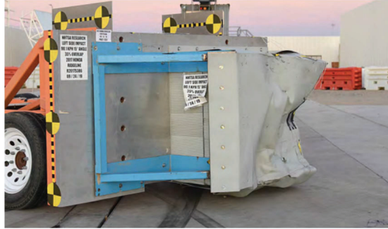
Figure 59 No honeycomb pulling apart from the Half V1
