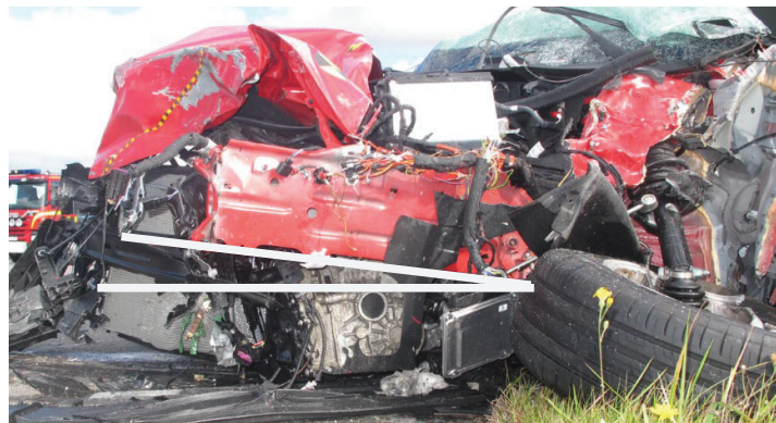
Figure 16: Front Longitudinal Deformation and Apparent Upward Rotation
