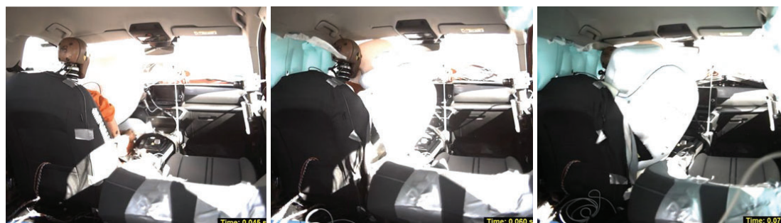
Figure 14. Occupant kinematics at 45, 60 and 75 ms into the crash.
