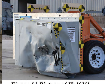
Figure 11 Picture of Half V1 honeycomb crush for the OMDB impacting Small production vehicle
