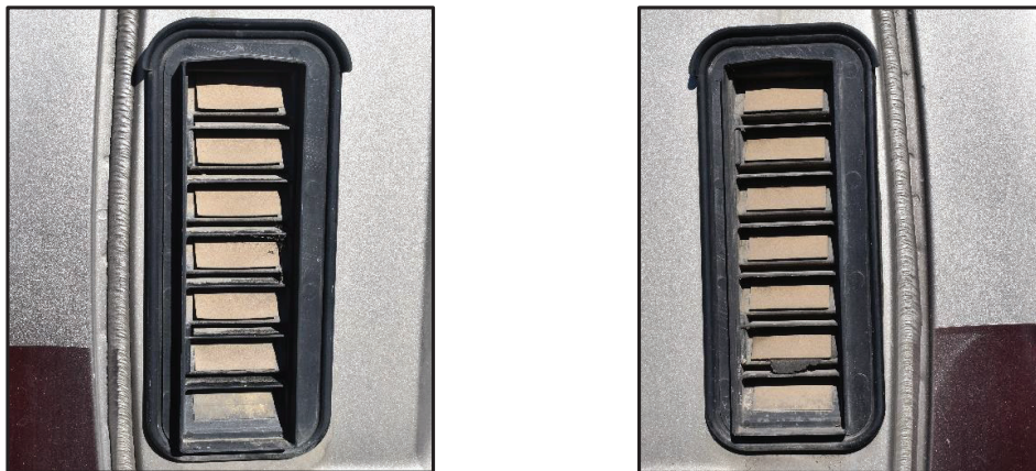
Figure 4: Exhauster vent 7a driver's side (Left) and 7b passenger's side (Right)
