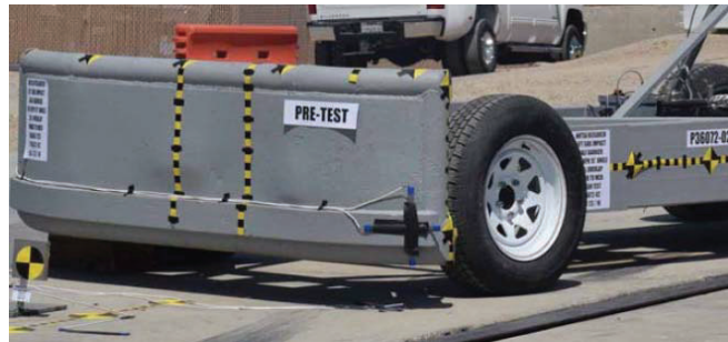
Figure 52 Picture of the moving contoured barrier (MCB)
