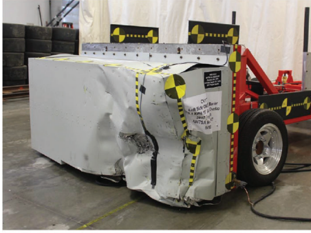
Figure 9 Picture of Full honeycomb crush for the OMDB impacting Small production vehicle
