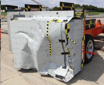
Figure 16 Picture of Half V0 honeycomb crush for the OMDB impacting Mid-size production vehicle
