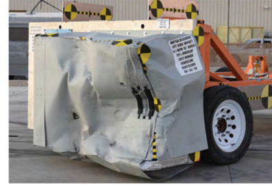
Figure 22 Picture of Half V1 honeycomb crush for the OMDB impacting Large PU production vehicle
