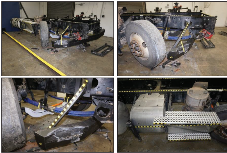
Figure 7. FUPS Sled Post-Test Photographs
