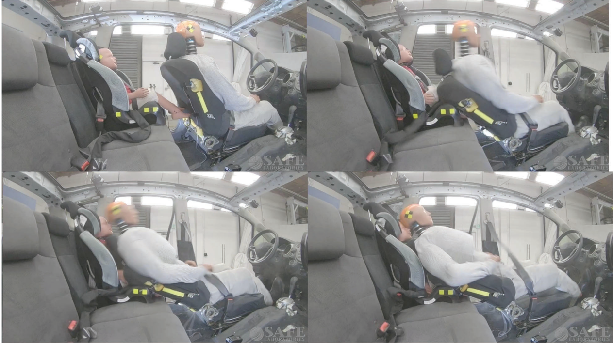
Figure 17: Sled test #2 occupant kinematics – heavy head to head contact.
