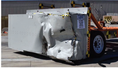
Figure 20 Picture of Full honeycomb crush for the OMDB impacting Large PU production vehicle
