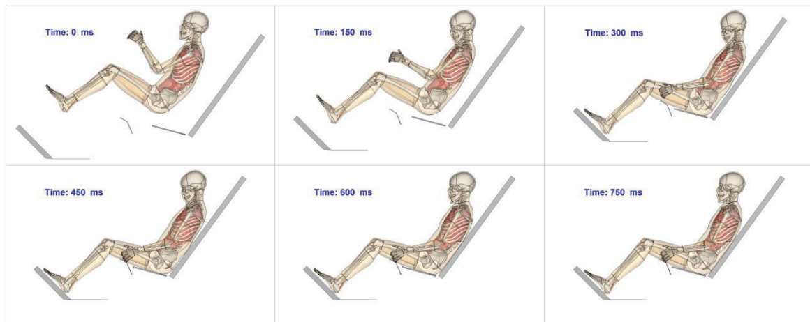
Figure 6: HBM positioning (pre)simulation. The environment elements (in grey) start 150 mm away from their original position and are repositioned during the first stage of the simulation. The last 300 ms are used to reach equilibrium in the model.
