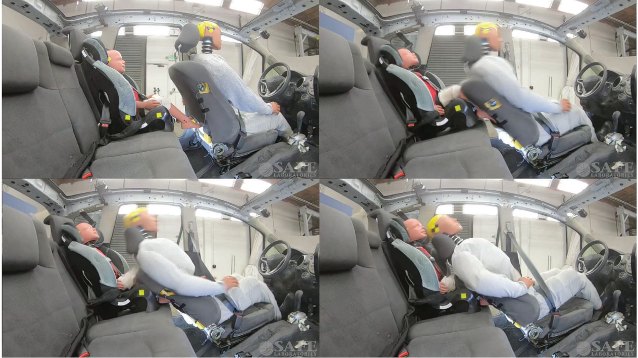
Figure 15: Sled test #1 occupant kinematics – no head-to-head contact.
