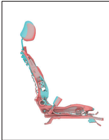
Figure 18: Sled test #2 seat deformation – minimal deformation.
