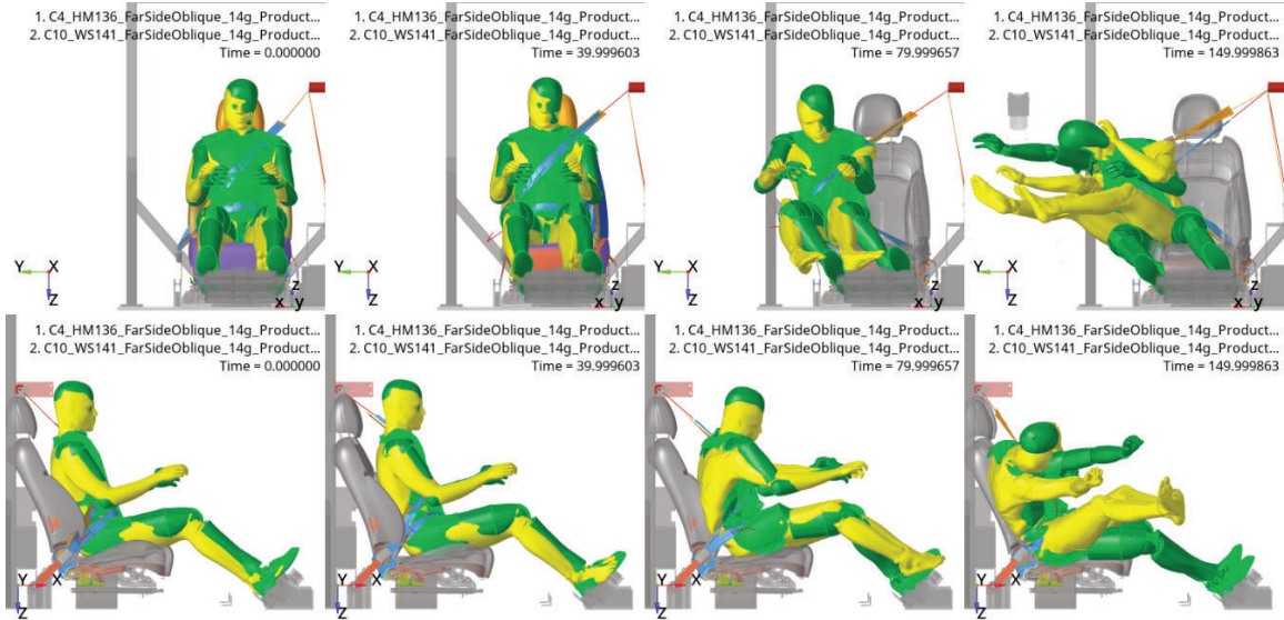
Figure 12. Snapshots of the kinematics of GHBMC M50-O model v6.0 from the simulated 14g 60 deg oblique far-side sled test with the production seat (case C4-HM136) compared to the paired THOR dummy case C7-TR139. (Green: the THOR dummy; Yellow: the HBM).
