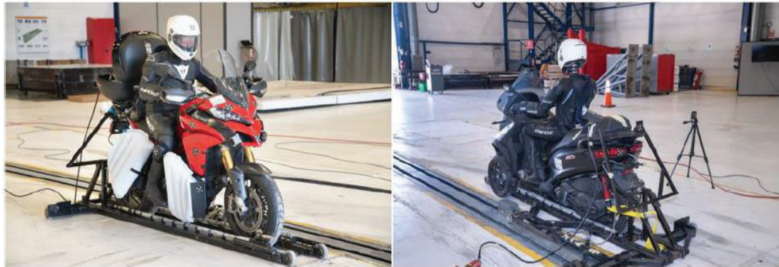
Figure 6. Images of the vehicle sled fitting the two types of motorcycle before the test
