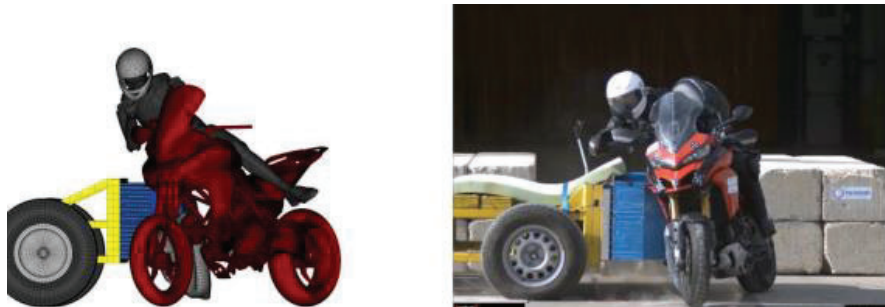
Figure 14. Impact with airbags: front view at 74ms
