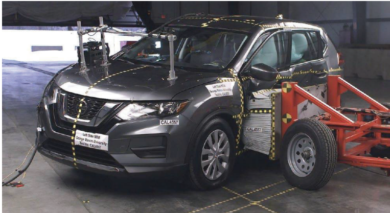
Figure 8. 2020 Nissan Rogue FMVSS No. 214-MDB full-scale test.
