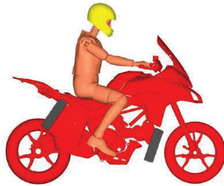
Figure 8. FE model of the Ducati Multistrada, with sitting Hybrid III and airbags (grey boxes)
